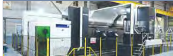
CNC Horizontal Lathe Machine For Turbine Rotors
