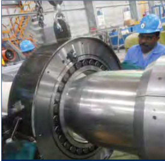
Assembly of Dredger Pump Bearing Block for Royal Boskalis Westminster N.V
